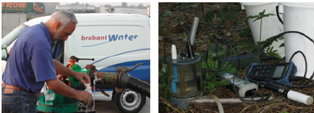
Figure 3.1. A water sample is taken from a water production well (left). Electrical conductivity and pH are measured in a water sample (right). Photos courtesy of water supply company Brabant Water, the Netherlands.
