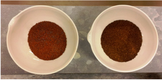
Figure 8. Color of heated Spannenburg material with CMC: left sample heated at 800°C, right sample heated at 500°C
