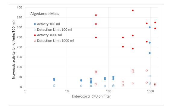
FIGURE 14. BACTCONTROL MEASUREMENTS OF 100 ML AND 1000 ML SAMPLES FROM AFGEDAMDE MAAS IN RELATION OF NUMBER OF CULTIVATED ENTEROCOCCI.
