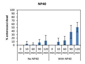
FIGURE 7. PERCENTAGE (%) OF DEAD (OR UNCULTURABLE) ENTEROCOCCI BACTERIA BY ADDITION OF NP40 TO THE NORMAL BUFFER. SHOWN IS AVERAGE (N = 4) WITH STANDARD DEVIATION. TEST WATER: WWTP EFFLUENT
