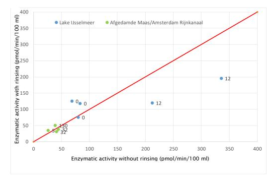
On the same water sample BACTcontrol analyses were performed with or without the rinsing step (20 ml MQ water; Figure 12).
