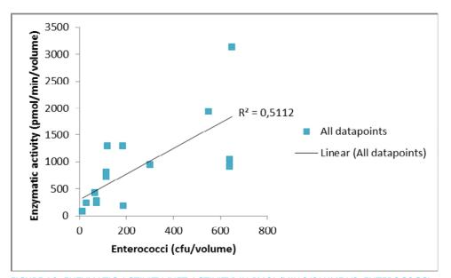
FIGURE 19. ENZYMATIC ACTIVITY (NET ACTIVITY) IN PMOL/MIN/VOLUME VS. ENTEROCOCCI CULTURE RESULTS IN CFU/VOLUME. SURFACE WATER OF PB. EPE WAS MEASURED WITH THE BACTCONTROL AND CULTURE AT THE SAME TIME. THE SAME VOLUME WAS USED IN BOTH METHODS.
