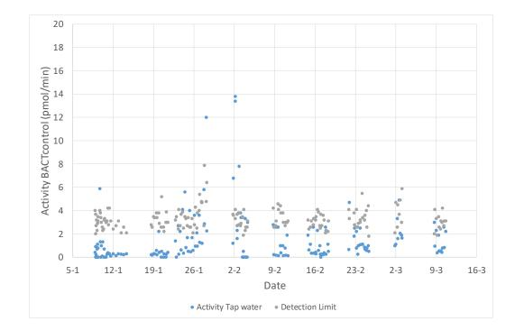
FIGURE 15. MEASUREMENT OF TAP WATER (100 ML)WITH THE BACTCONTROL ENTEROCOCCI ASSAY AT LOCATION HAARLEM DURING THE WEEKENDS.
