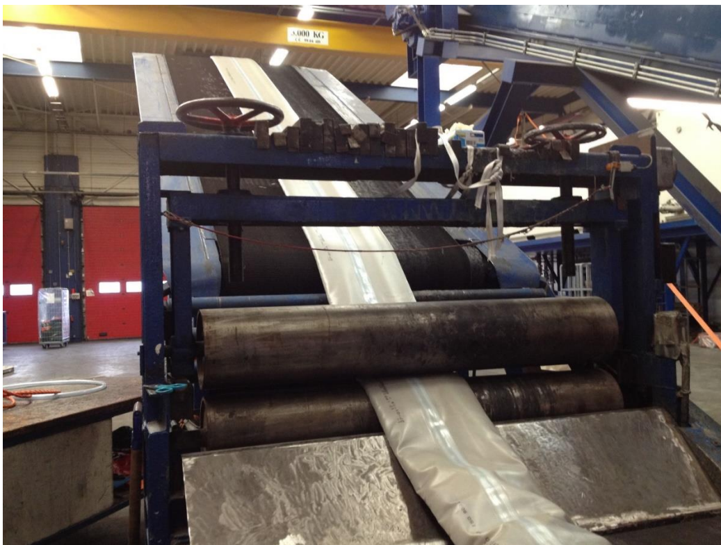
Figure 1 Impregnating a liner with resin.
