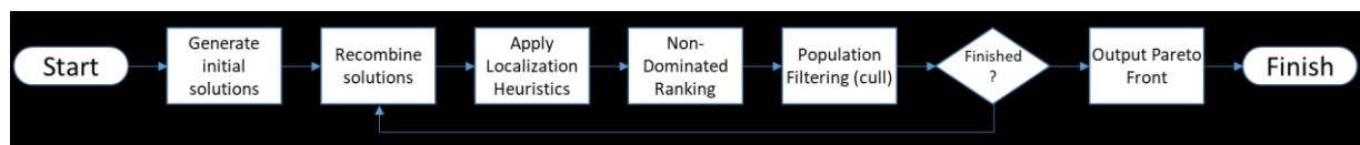
Figure 9. Flowchart of the leak localization algorithm
