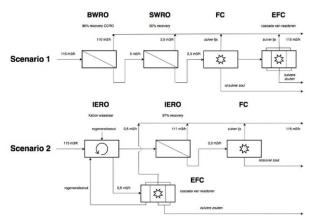
Total concepts envisaged for the production of water of high quality from brackish groundwater in which solid-phase residual streams are generated
