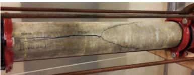
Asbestos-cement pipes taken from the field are, under controlled conditions, subjected to internal pressure until bursting to get an insight into their residual strength following many years' usage.
