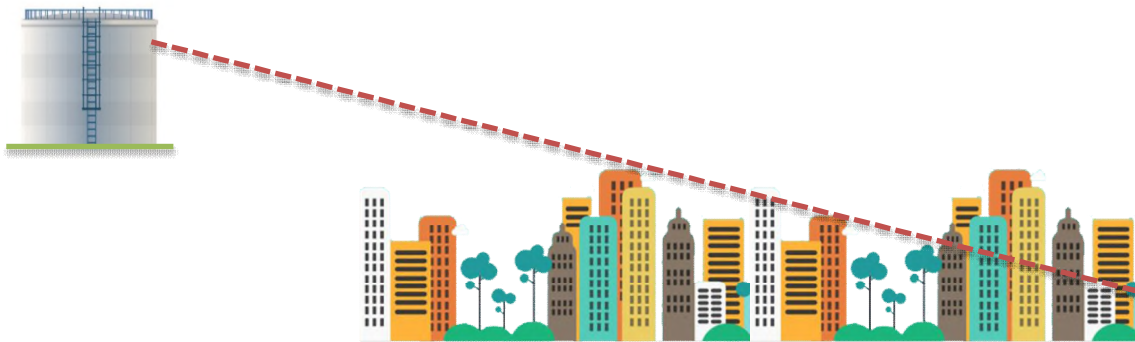
Figure 3. Piezometric line in Pressure Driven Method
