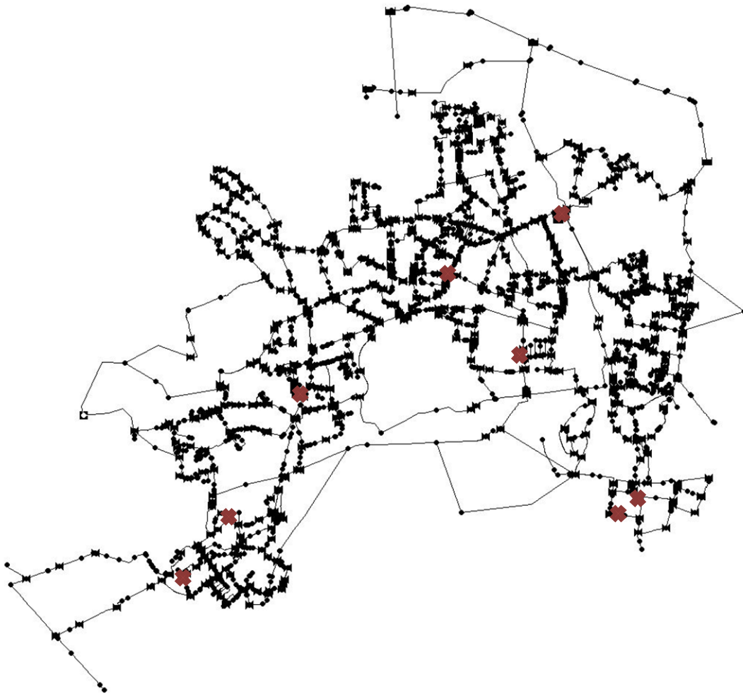
Figure 32. Combination of closed valves 1
