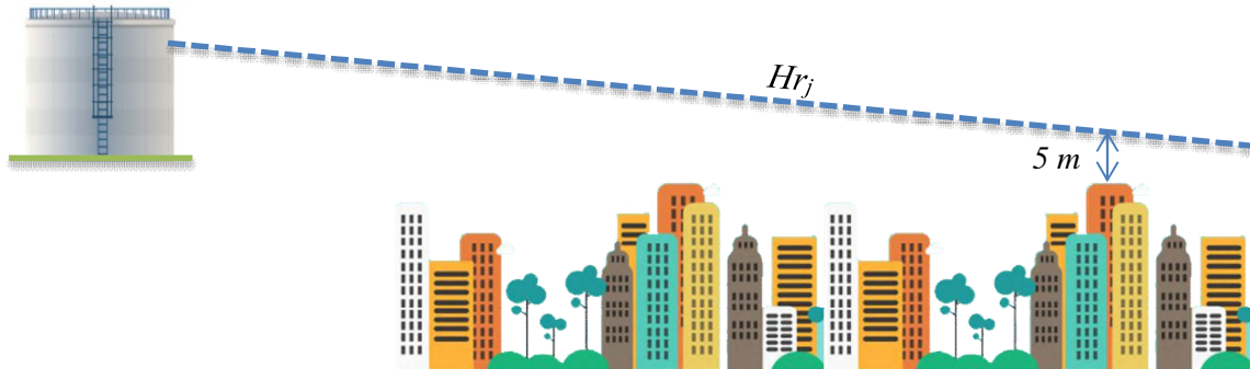
Figure 2. Piezometric line in Demand Driven Method
