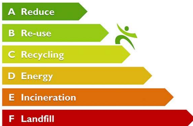
Figure 6 Dutch waste management adopted the principles outlined in this “ladder van Lansink” embedded in Dutch law since 1993. It provides a priority ladder for solid waste management.
