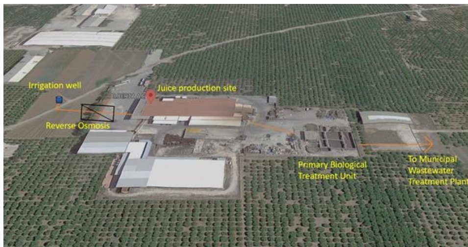
Fig. 11 Alberta water system before Ultimate
