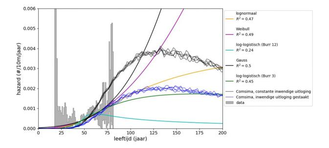
Five probability distributions that are frequently used to describe and extrapolate failure behaviour, fitted to the failure data from Brabant Water. Also shown, for comparison, are two predictions of the failure behaviour with the Comsima physical model. In this manner, a choice for a particular distribution can be supported by the physical knowledge behind Comsima.
