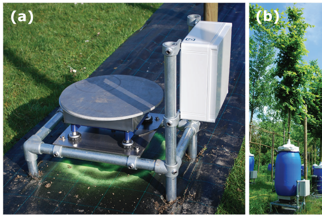
FIGURE 1 Experimental set up: Weighing balance (a), tree on balance with white rain cape (b)
