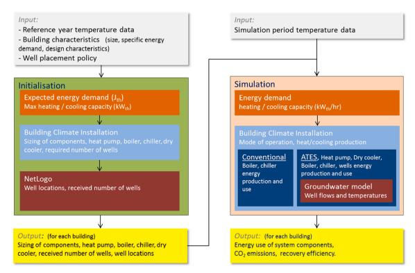
Fig. 4. Schematic representation of the simulation framework of the different components of the used modelling system.
