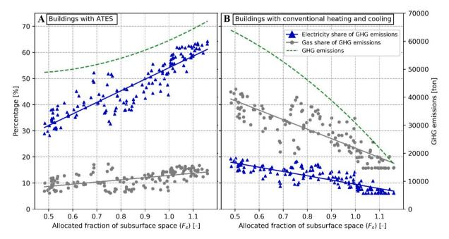
Fig. 15. Share of total GHG emissions due to buildings with an ATES systems (left) and building with conventional buildings (right). With higher allocated fraction of subsurface space (F<sub>s</sub>) the share of emitted GHG emissions increases for ATES and decreases for conventional buildings.
