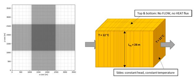
Fig. 10. Left: top view plot of the horizontal discretization. Right: conceptual model of the 3D grid.
