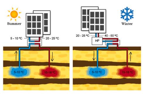
**Fig. 1.** Basic working principle of a low-temperature (LT) ATES-doublet. Right: In winter, buildings are heated with a heat pump (HP) which extracts heat that was previously stored in the warm well. This creates cooling capacity which is stored in another well in the subsurface. This cooling capacity is used in summer (left) to cool the building, by storing the excess heat in the warm well. From: Bloemendal et al. [6].
