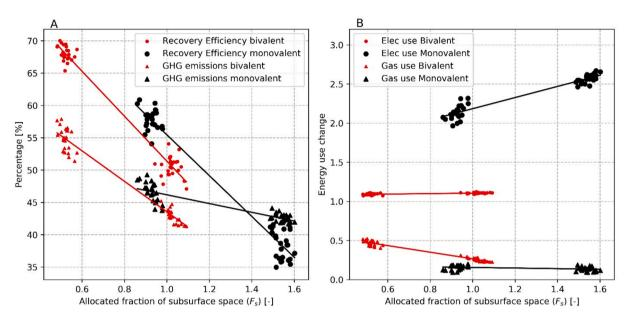
Fig. 19. Monovalent and bivalent simulation results. A: recovery efficiency and GHG emissions reduction. B: electricity and gas use.
