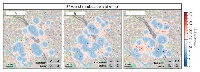
Fig. 12. The effect of different well placement policies based on the relative thermal radius distances between same ( $D_s$ ) and opposite ( $D_o$ ) thermal well types on temperature distribution in the storage aquifer in the end of the winter of the 5th year of the simulations for 1 random model realisation for 3 different placement policies. From A-C density well placement density increases with decreasing  $D_s$  from 2 to 0.5 times and  $D_o$  from 3 to 2 times the thermal radius.
