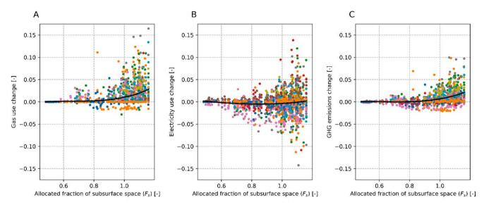
Fig. 17. Gas use, electricity use and GHG emissions change for individual ATES systems in different model realisations due to increasing levels of aquifer utilization (F<sub>s</sub>) compared to the lowest aquifer utilization model run that resulted in the maximum number of desired wells for each individual ATES system / building. The solid line indicates the average change of the ATES systems at given F<sub>s</sub>.
