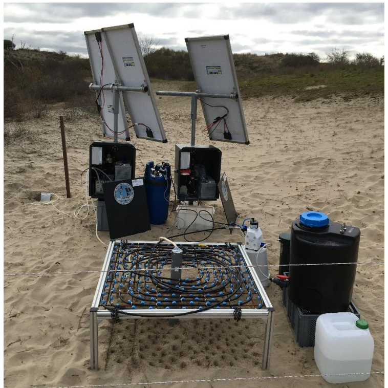
Figure 2 Field equipment set-up in the tracer and faeces trials. Solar panels provided power for the groundwater and the air-pumps.
