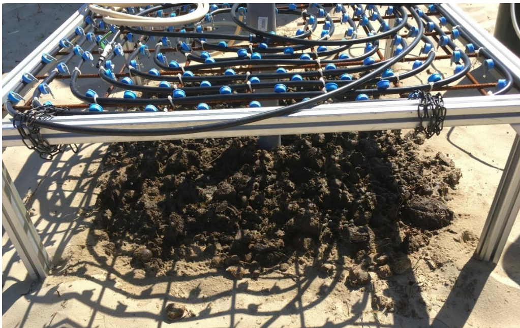
Figure 3 Set up of faeces within the perimeter of the rain equipment.
