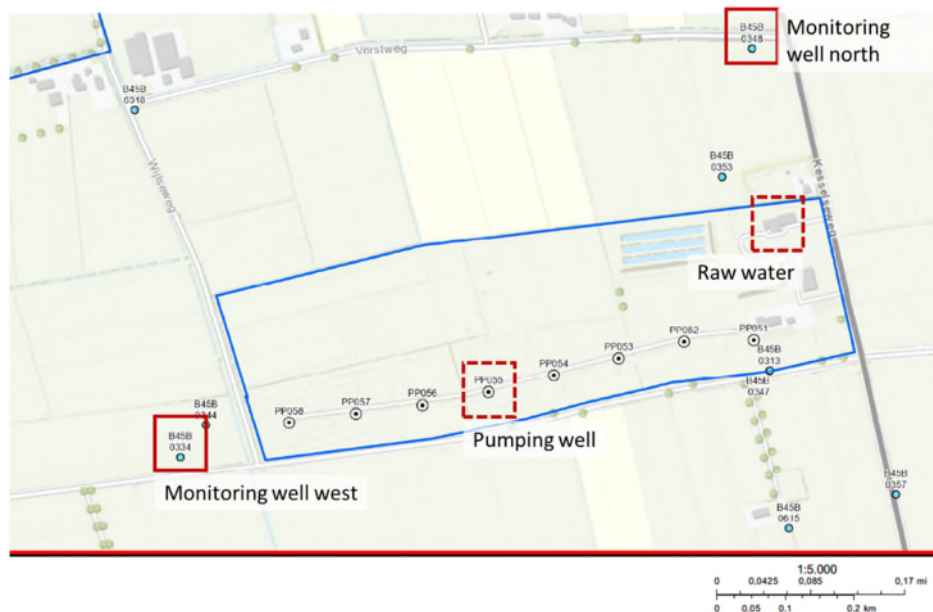
Figure 1: Overview of the case study site with the 4 measured locations. Dashed line indicates locations where the developed flow cells were employed. For each monitoring well a deep and shallow screen was used to be measured, resulting in a total of 4 monitoring well measurement locations.
