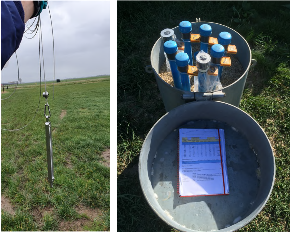
Figure 14: Left: Passive sampler going into a groundwater well for sampling. Right: finished installation of the undep and deep passive sampler (sealed steel rings).
