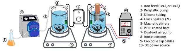
Fig. 2. Fe dosage bench scale setup, with chemical dosage (left) and electrochemical dosage (right).
