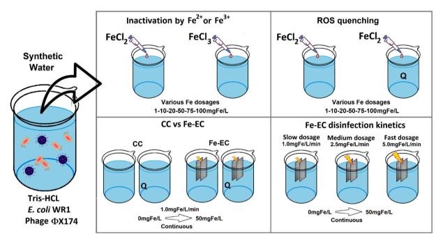
Fig. 3. Schematic description of the four Fe disinfection experiments. Letter "Q" indicates the beaker was dosed with an ROS-Quencher. Pipette represents singleevent chemical dosage, while the arrow represents continuous dosage either by CC (FeCl<sub>2</sub> solution dosed with peristaltic pump) or Fe-EC (Fe dosed electrochemically under a constant current).
