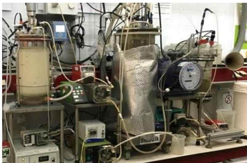
Figure 7. Laboratory scale AnSBR (Sparthane™) set-up.
