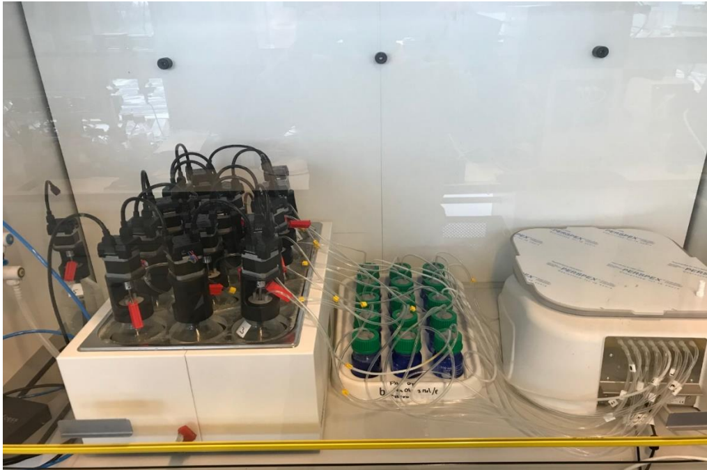
Figure 11. Lab-setup for batch anaerobic batch tests (AMPTS).
