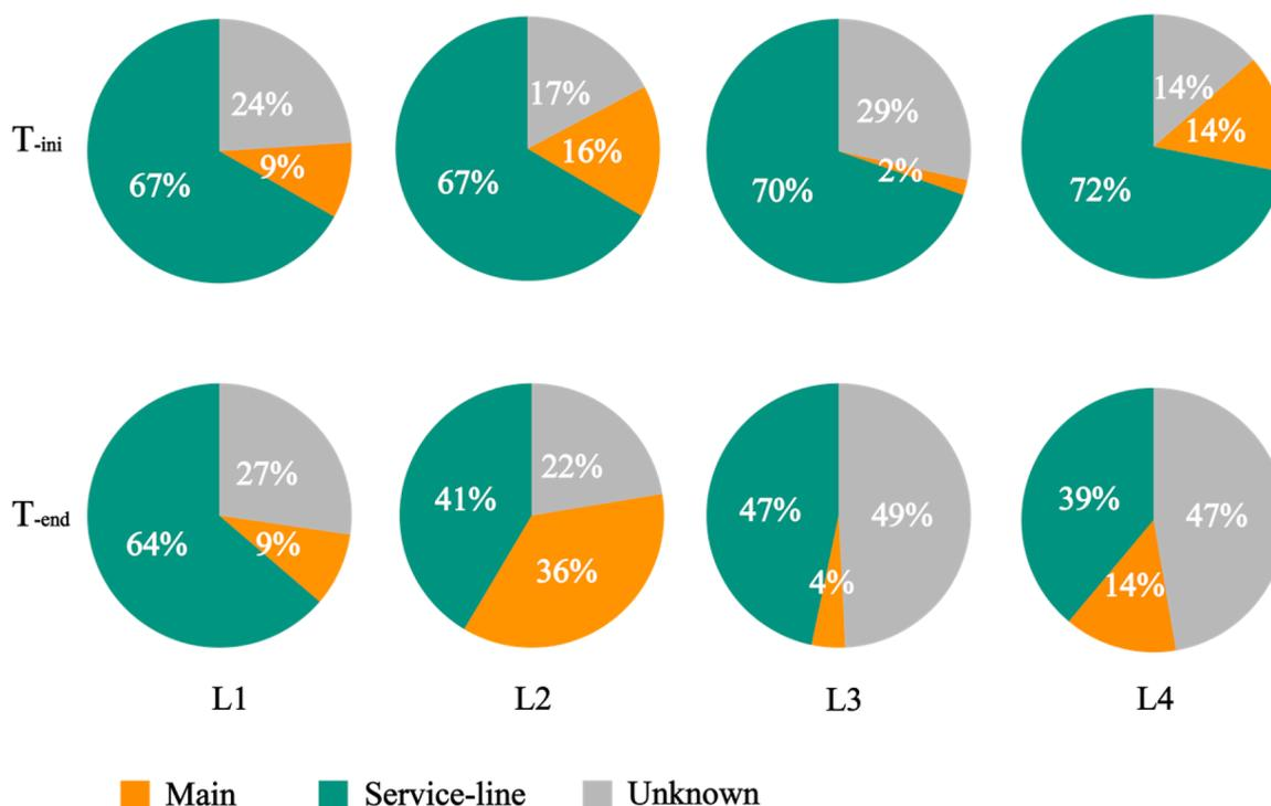
Fig. 5. Origination of filter-bag particles calculated by SourceTracker2-based microbial community fingerprints at T<sub>mid</sub> and T<sub>end</sub>. The results are presented by the filter bags collected from each location (Table S8).
