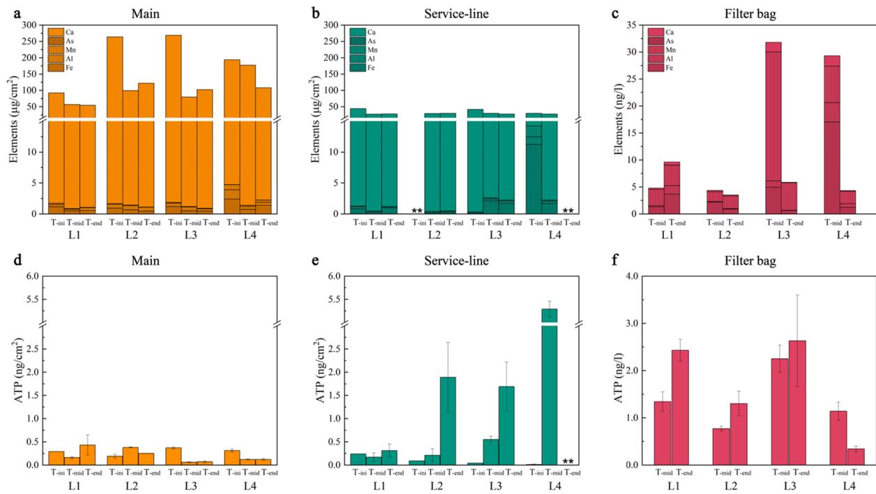
**Fig. 2.** Metal elements of Fe, Al, Mn, As, and Ca (a, b, c) and ATP (d, e, f) of the biofilms sampled on main and service line pipes and particles collected on the filter bags at 4 locations in a DWDS at T<sub>ini</sub>, T<sub>mid</sub> and T<sub>end</sub>. The ATP and elemental composition corresponding to each location are provided in Tables S3, S4, and S5. Elemental and ATP concentrations for filter bags was normalized by the volume of water flowing through.
