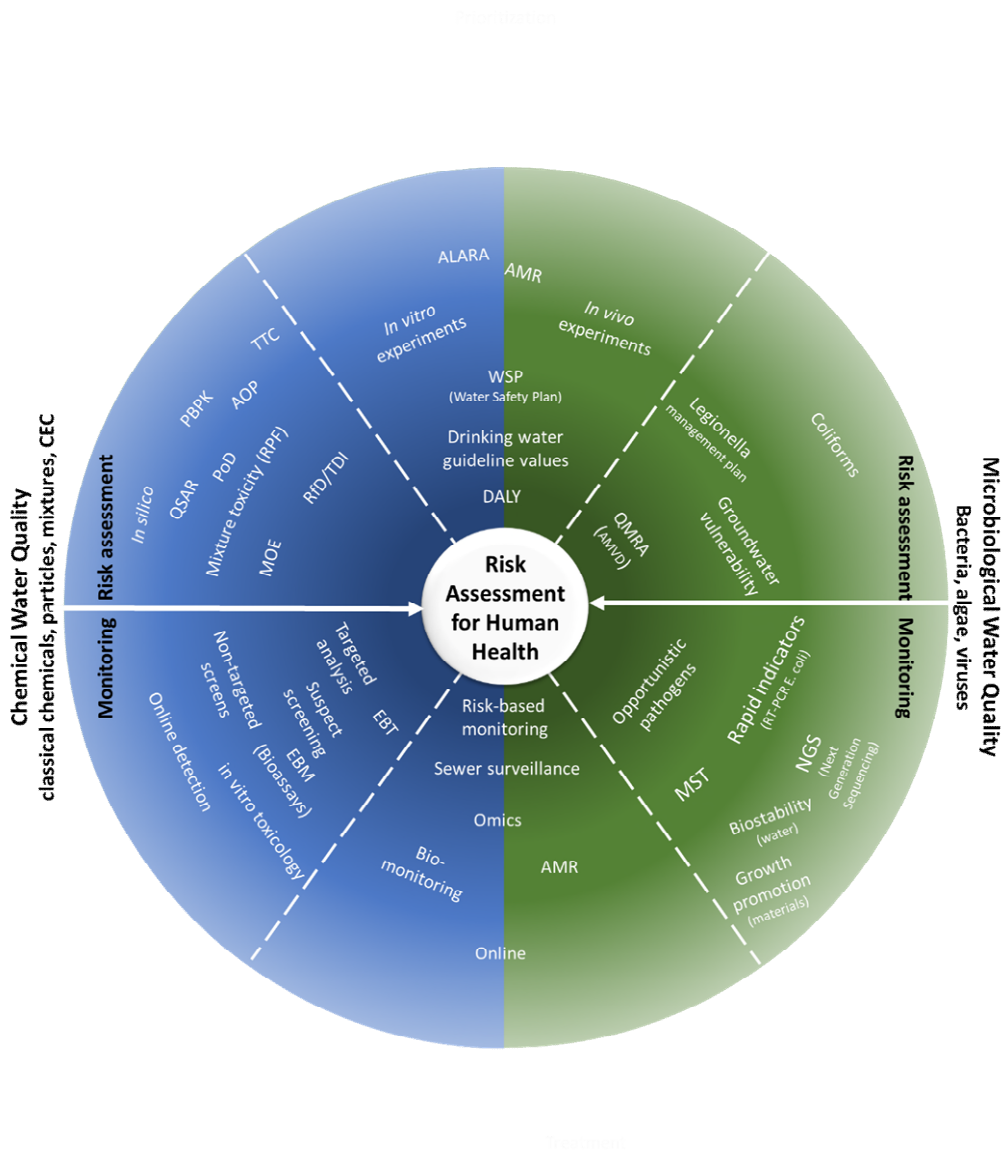
Figure 1 Overview of the chemical and microbiological water quality and risk terminology in drinking water (not exhaustive). The parameters are divided in monitoring parameters (bottom half) and risk assessment parameters (top half). Terms between the dashed lines refer to both chemical and microbiological aspects. Terms closer to the centre provide more quantitative information on human health risks.
