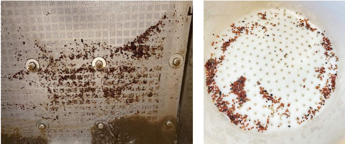
Figure 36 A. Retention of the anammox granules by the fine sieve 1mm. B. Determination of anammox granule concentration on day 196
