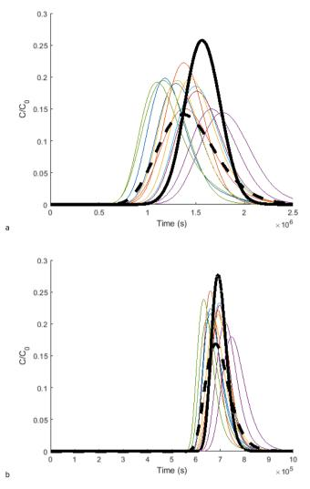
**Fig. 3.** Breakthrough curves for all 12 realizations of the heterogeneous soil, the heterogeneous average (bold dashed line), and the homogeneous soil (bold solid line), for (a) MM (steady-state flow) and (b) MH (transient flow) infiltration scenarios respectively, for scenario C1 with contaminant input  $C_0 \gg K_{A,C}$ .
