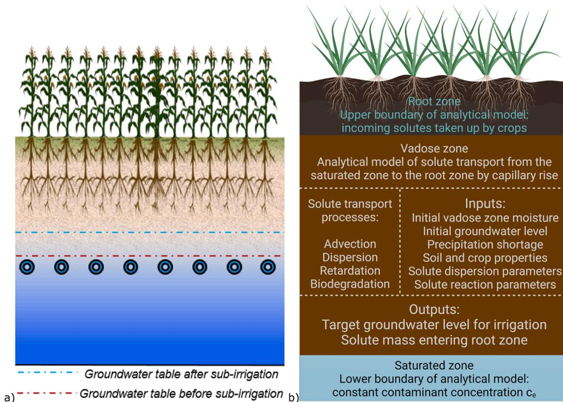
Fig. 1. (a) Conceptual illustration of the phreatic zone irrigation system. (b) Conceptual overview and illustration of the analytical model and a list of the processes it considers, with inputs and outputs.
