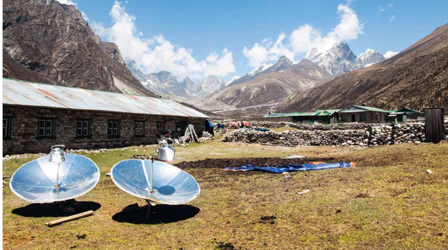
Solar boilers are used in the Himalayas to cook food and boil water
