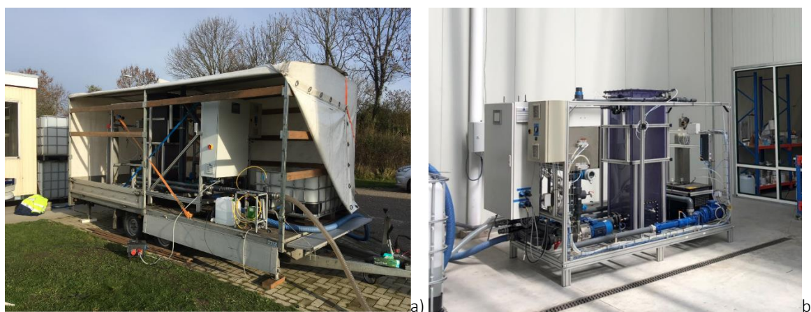
Figure 7- PureBlue Ozone pilot at Walcheren with KWR dosing system (a); Ozone pilot at PureBlue facilities at Kapellebrug, 2022.
