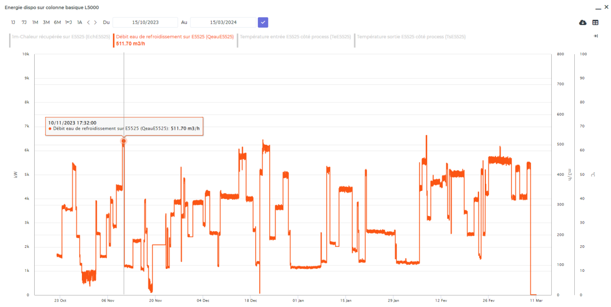
Figure 77 Parameter “Cooling water flow rate on E5525, one of the three parameters displayed in the widget in Figure 76
