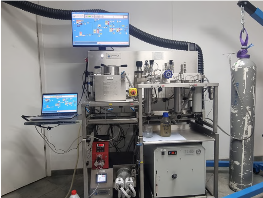
Figure 38 Subcritical/Supercritical Extraction Equipment
