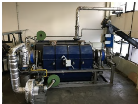
Figure 12. Rotary kiln for slow pyrolysis (PYROCK).
