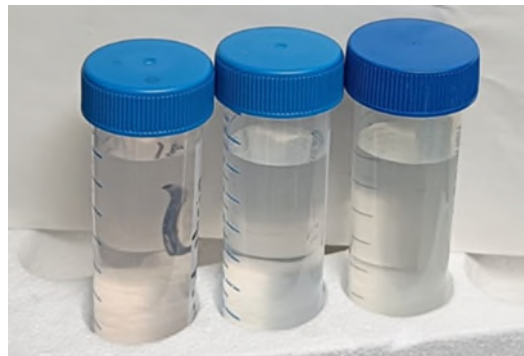
Figure 73 Photos of samples of the ammonium sulphate solution recovered from the scrubber.
