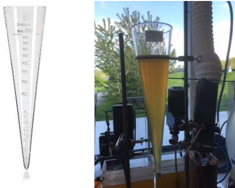
Figure 3-4 Photo of an Imhoff flask, empty and filled within the experiments.
