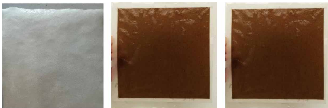
Figure 1 | Images of the nonmodified (left) and crown ether–modified membranes (15C5 (middle) and 18C6 (right)). All membranes were of size 11 \times 11 \text{ cm}^2 .
