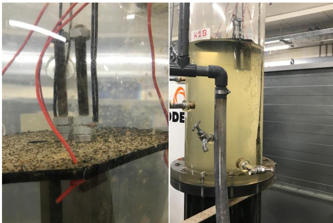
Figure 4 EC dosing cassette on pilot sand filter column.
