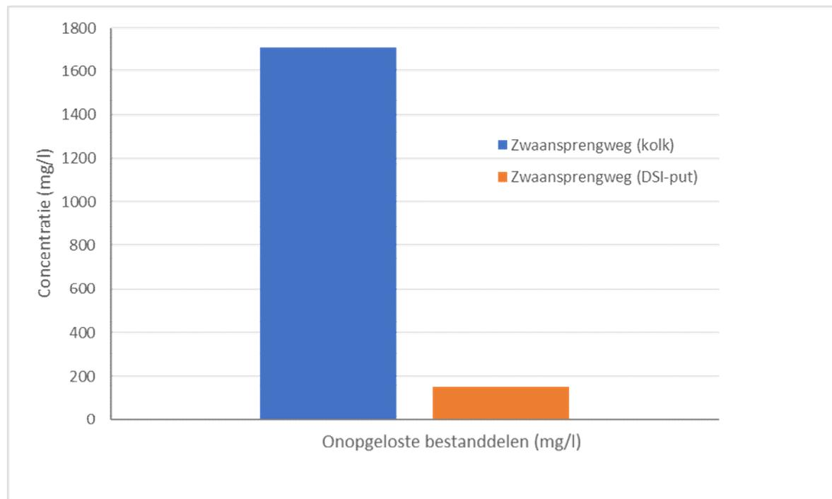
Figure 20: Example of removal of suspended solids using a 'HWZI' high-rate sand filtration system (source: municipality of Apeldoorn). With blue the concentration suspended solids before and orange the concentration after pretreatment.
