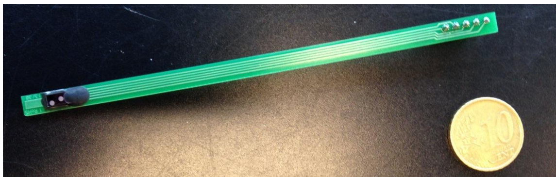
Figure 2: Picture of provided pH sensors from Holst/Imec. On the left, the micro-fabricated sensor chip is visible with the two different (circular) electrodes.
