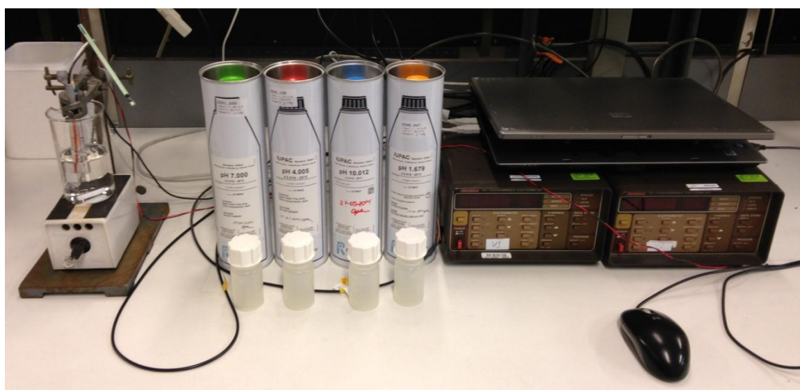
Figure 3: Batch Measurement setup with beaker, sensors, read-out electronics and PC.
