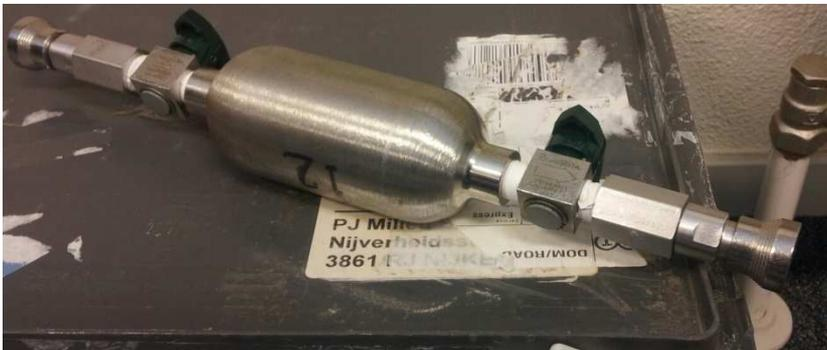
Figure 2: Stainless steel cylinder used for gas sampling.
