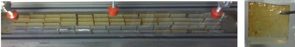
Figure 4.4. BPU loaded with new PVC plates and biofouled PVC plates after 12 days of cultivation and a biofilm sample after 29 days of incubation
