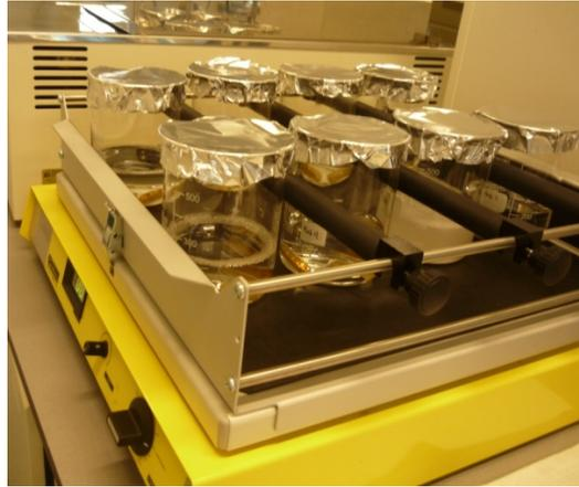
Figure 3.6. Picture of the orbital shaker with the cleaning test beakers
