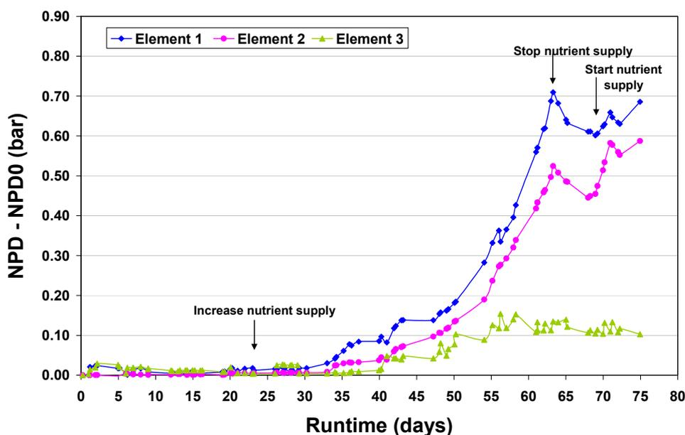
Figure 4.23. Normalized pressure drop difference for each of the elements evaluated on the spiral-wound membrane setup
