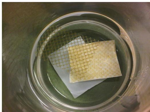
Figure 4.22. RO membrane sample in the laboratory cleaning test
