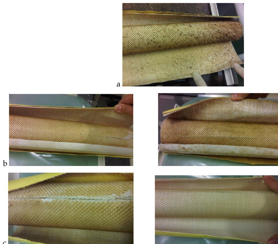
Figure 4.24. Autopsy images of the biofilm formation on a) SWM 1 (feed side), b) SWM 2 (left, feed side; right, end side) and c) SWM 3 (left, feed side; right, end side)
