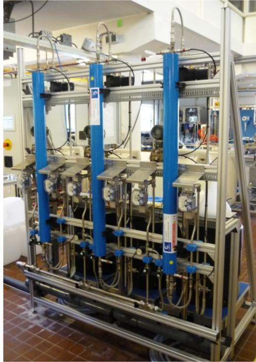
Figure 3.4. Spiral-wound membrane system setup.
