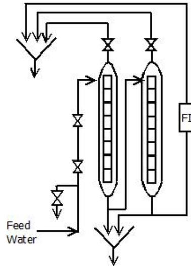
Figure 3.3. Biofilm formation monitor picture and scheme
