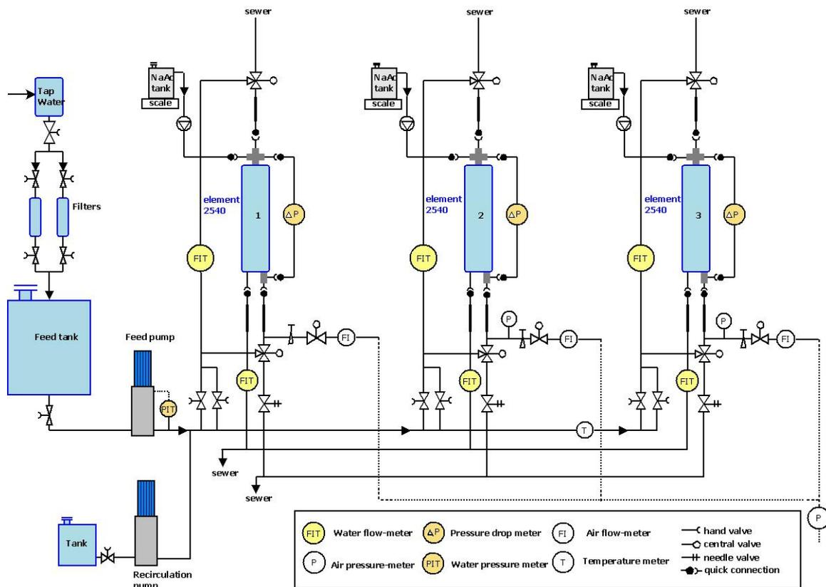
Figure 3.5. Spiral-wound membrane scheme
