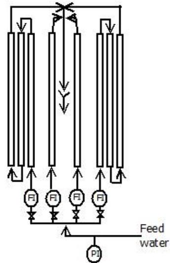
Figure 3.2. Biofilm formation setup picture and scheme
