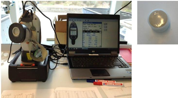
Figure 6. Handheld XRF analyser (left) and soil samples (right)
