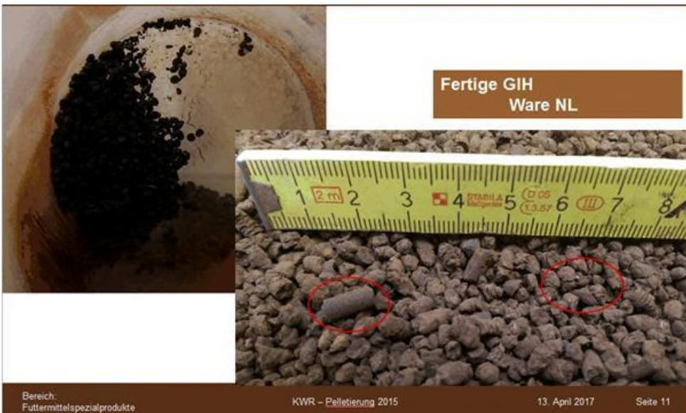
FIGURE 10 GIH-PELLETS PRODUCED BY EXTRUSION.
