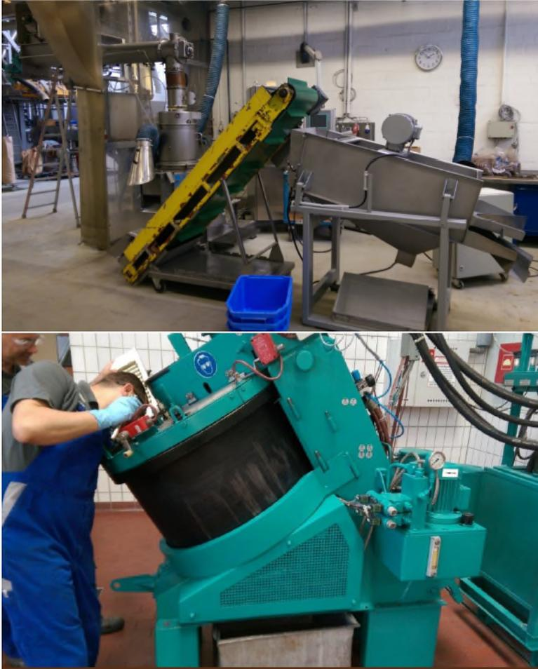
FIGURE 12: PELLET PRODUCTION AT AGRAVIS. UPPER FIGURE: EXTRUSION PROCESS, APPLYING PRESSURE. LOWER PICTURE: INTENSIVE MIXING PROCESS.
