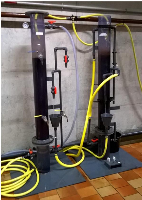
FIGURE 30 PILOT COLUMNS FILLED WITH GIH-PELLETS AT PRINSENBOSCH.
