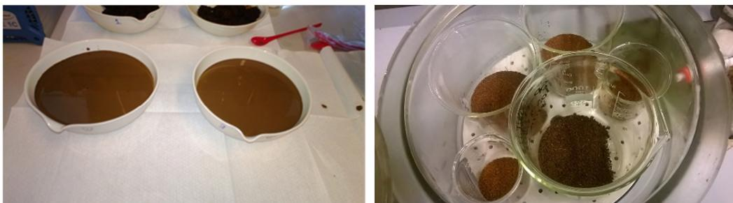
FIGURE 5 DRINKING WATER TREATMENT RESIDUALS BEFORE AND AFTER PROCESSING INTO PELLETS AT LABORATORY SCALE.
