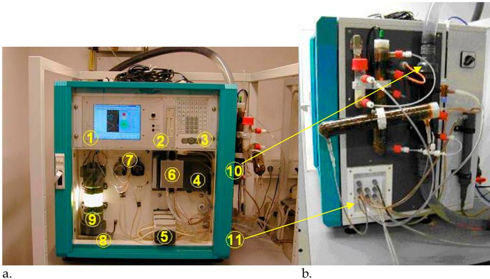
Figure 1.1 Components of the *Daphnia*-toximeter ; a. front view, b. side view.
