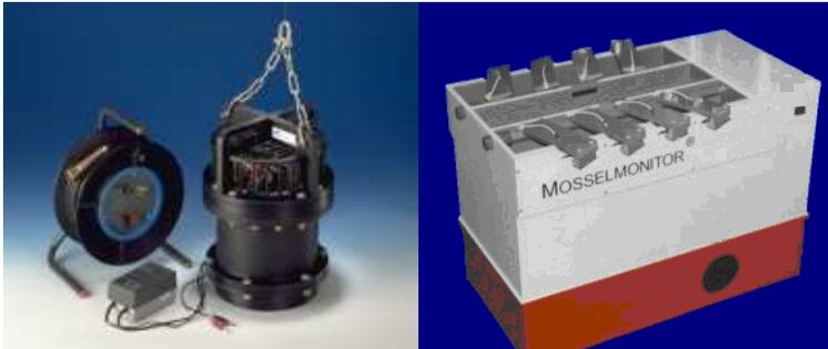
**Figure 1.1** The MOSSELMONITOR® (left: *in situ* (submersible) and right flow-through instrument)
