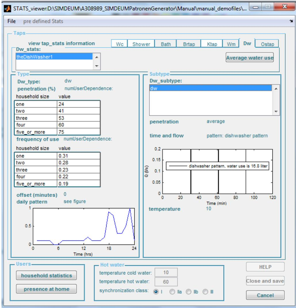
Figure 4-7 View .stats-file with data for dishwasher in demo\_house\_manual\_week.stats.
