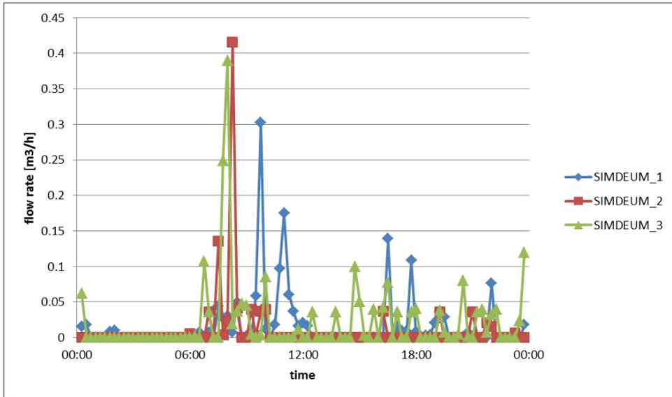
Figure 8-3 Example of demand patterns for three houses in Excel file, time step is 900 seconds and flow rate unit is m<sup>3</sup>/h.
