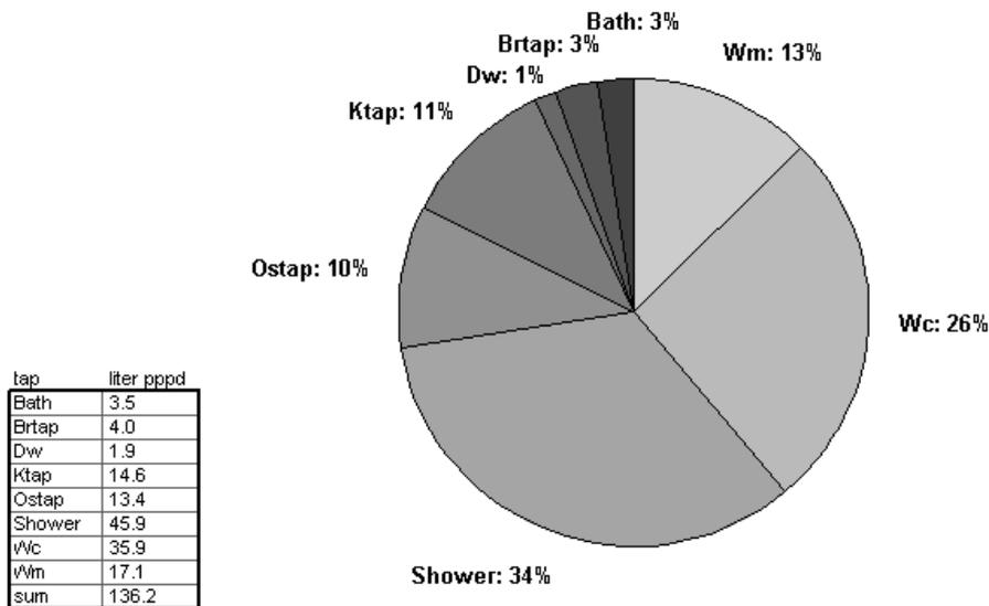
Figure 4-8 Average water use of the building/household defined in `demo_house_manual_week.stats`.
