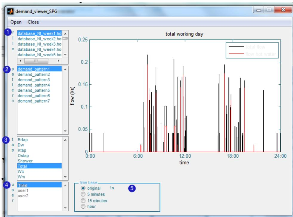
Figure 7-2 The demand viewer of SIMDEUM Pattern Generator, that shows the demand patterns of cold and hot water in different houses during different days.
