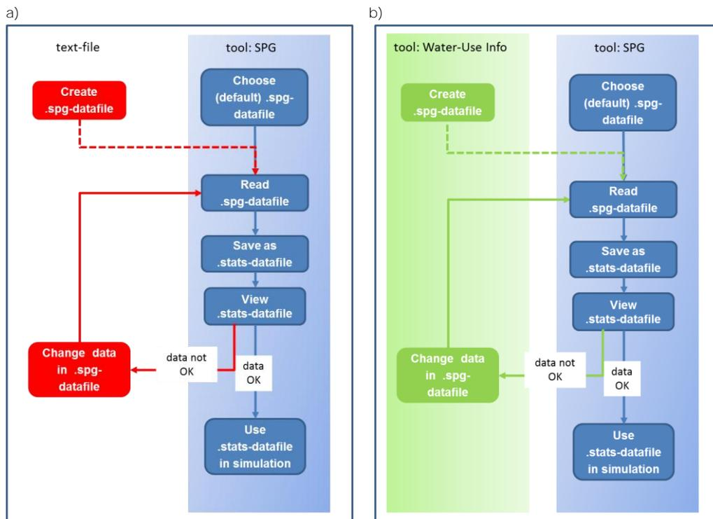
Figure 5-1 Procedure to create a spg-file starting from a default or demo spg-file or default stats-file: a) using a text-file and b) using Water-Use Info in Watershare®.
