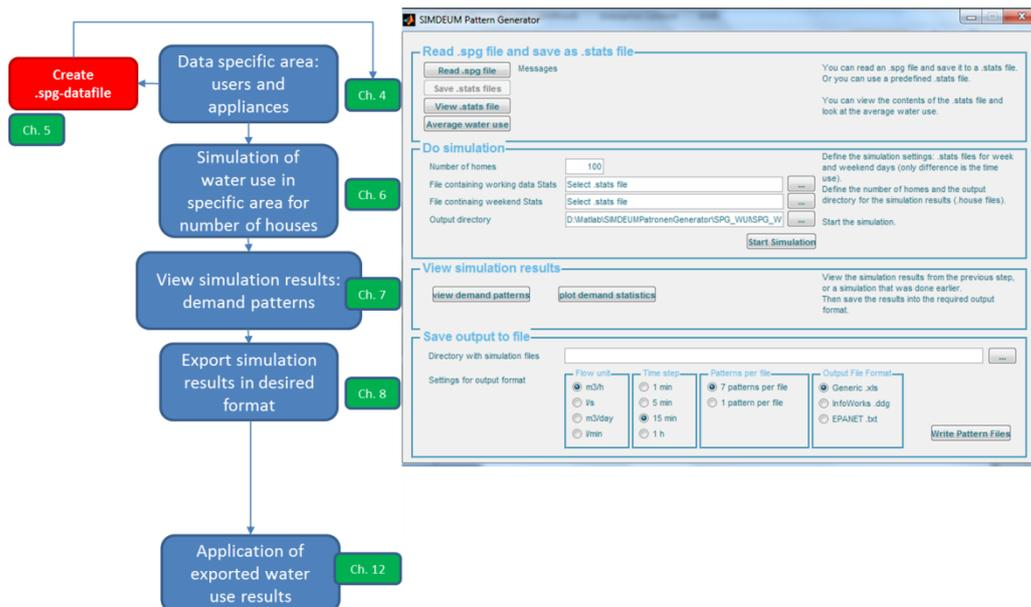
Figure 3-1 Structure of the SIMDEUM Pattern Generator for residential buildings and the corresponding chapters of this manual.
