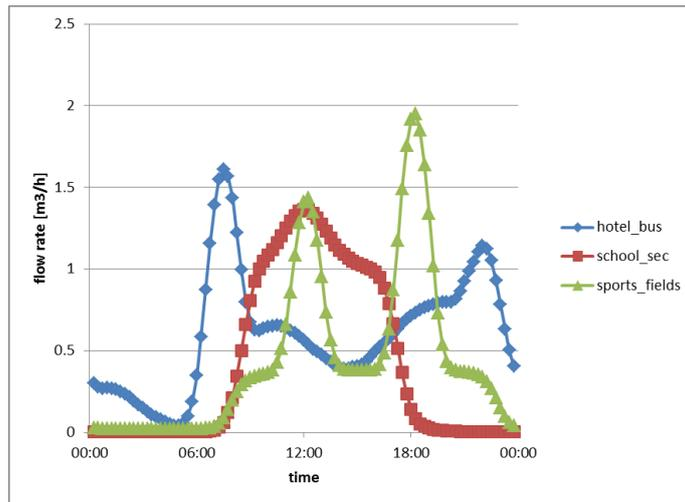
Figure 11-3 Example of demand patterns of three non-residential buildings, a business hotel, a secondary school and sports fields in Excel file, time step is 900 seconds and flow rate unit is m<sup>3</sup>/h.
