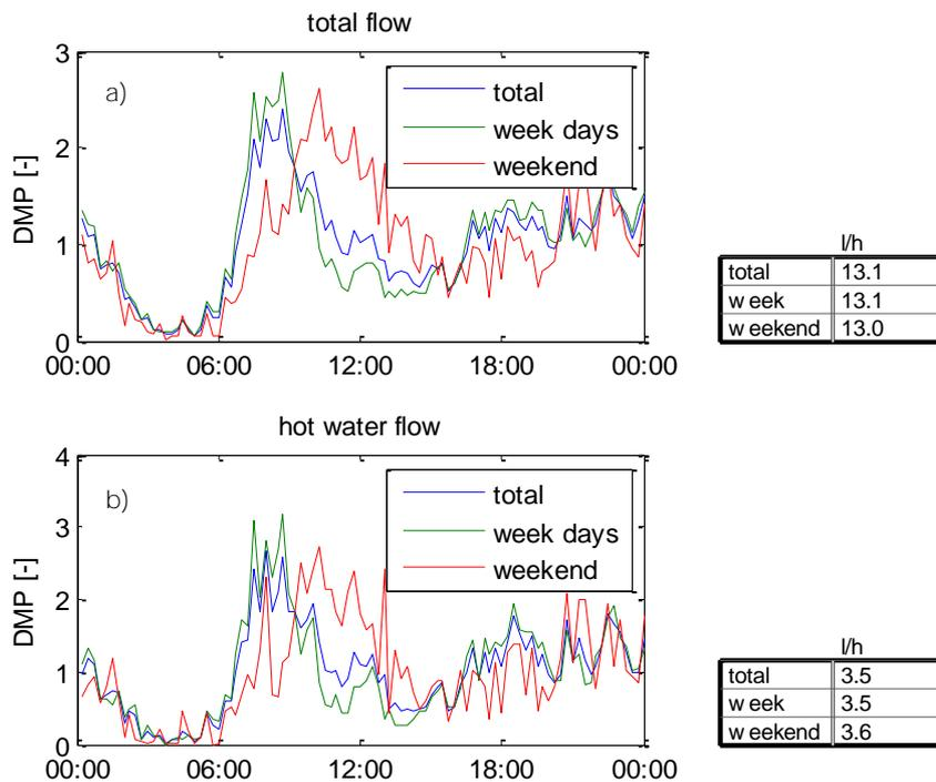
Figure 7-3 Average normalised demand patterns for total number of houses, for all days (blue), during week days (green) and during weekend days (red): a) for total (cold and hot water) flow and b) for hot water flow. The tables give the average water use per house in [l/h].
