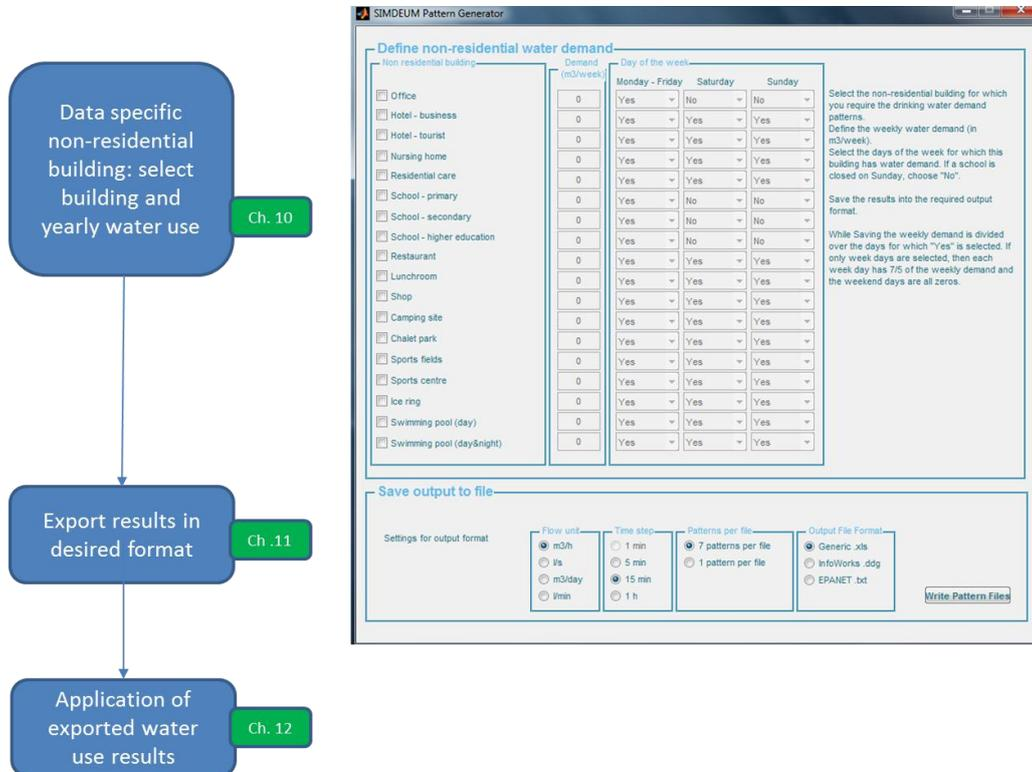
Figure 9-1 Structure of the SIMDEUM Pattern Generator for non-residential buildings and the corresponding chapters of this manual.
