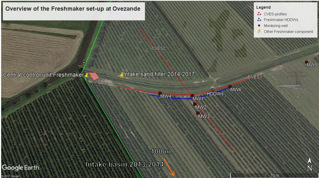
Figure 2.8: Plan view of the Freshmaker set-up at the Ovezande pilot site. (HDDWs = horizontal directional drilled wells, CVES = continuous vertical electrical soundings, MW = monitoring well).
