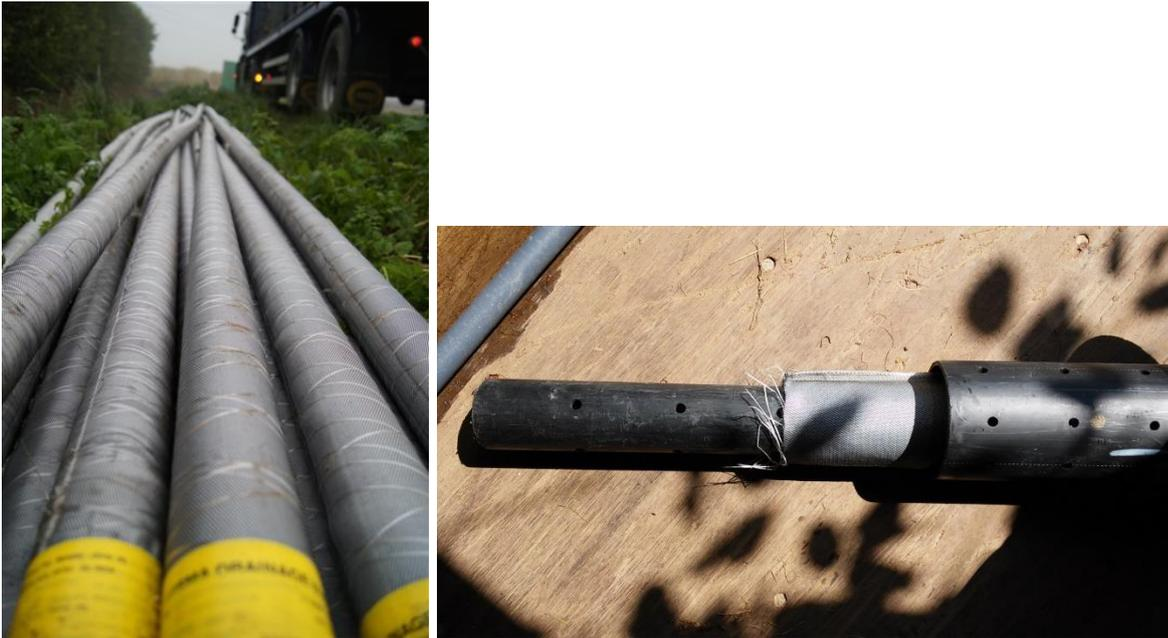
Figure 9.2: Left: well type used at the Ovezande reference site: HDPE wrapped in Geotextile (75 mm). The deeper HDDW2 was protected by a 125 mm perforated HDPE pipe (right)
