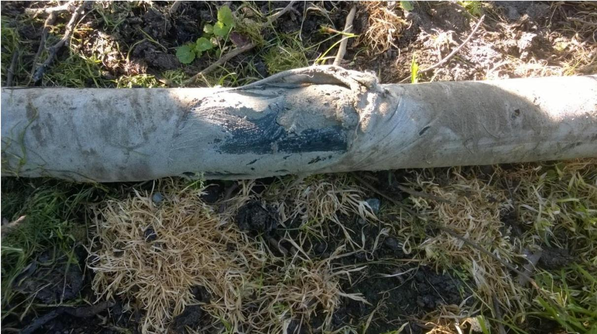
Figure 9.14: Damaged textile around the HDDW Groede, creating inflow of sand.
