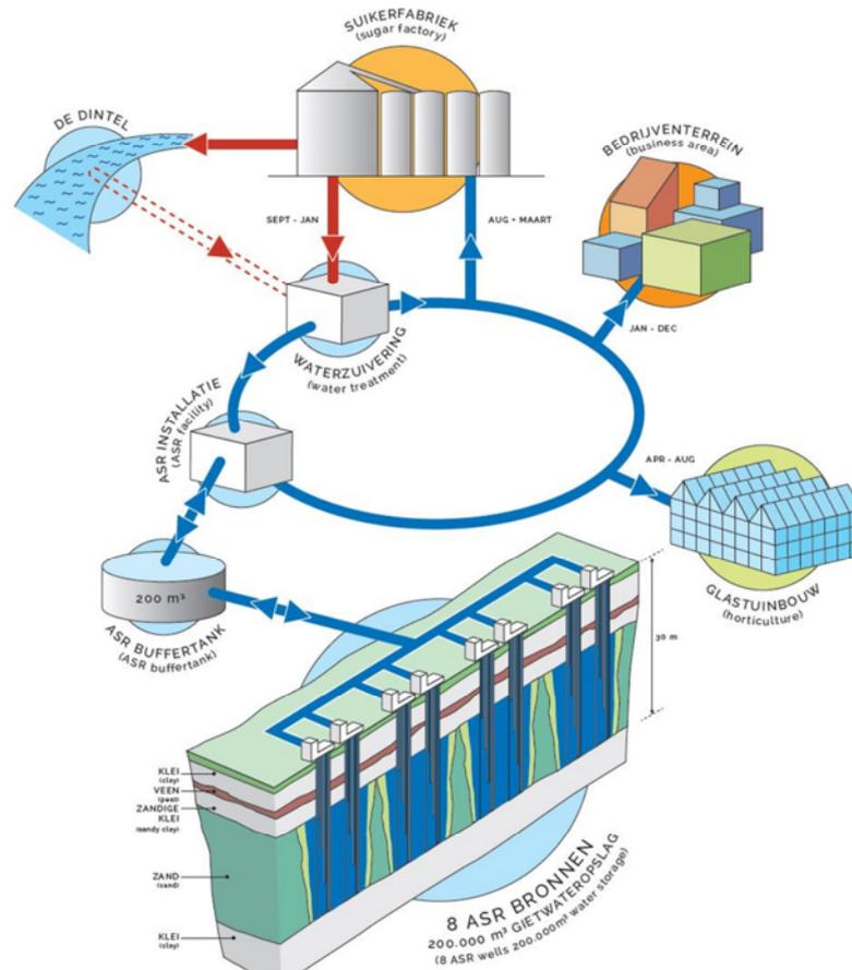
Figure 3.4. Set-up of the sustainable water supply system in Dinteloord (Zuurbier et al. 2018),
