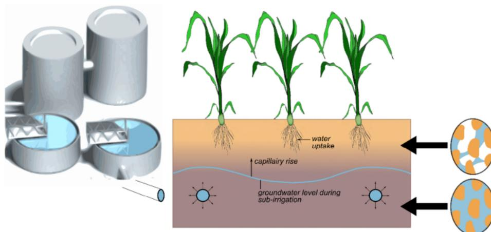
Figure 3.2: Schematic of Haaksbergen irrigation site. Subirrigation via drains with continuous water supply, with which the water table and the soil moisture regime could be controlled actively.
