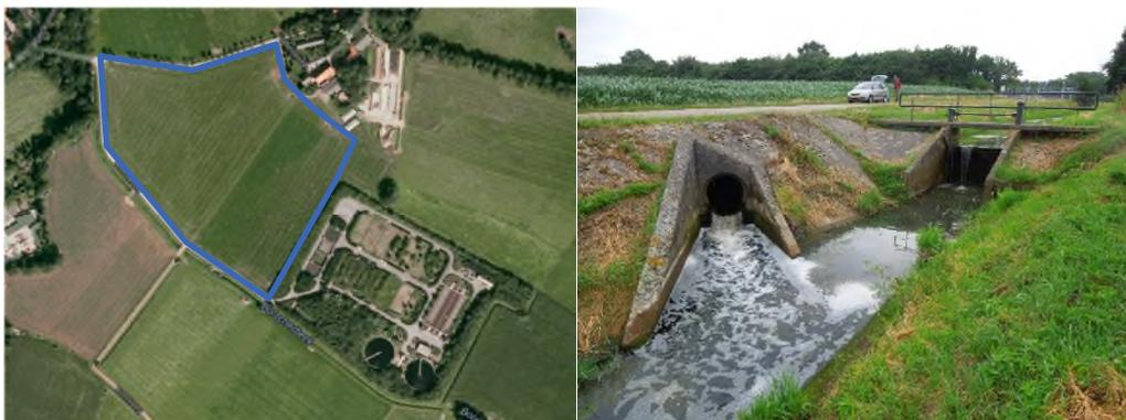
Figure 4.1: Left: view of the STP, Bolscherbeek and the pilot field in which effluent is used for subsurface irrigation. Right: The Bolscherbeek is supplied with effluent from the Haaksbergen sewage treatment plant. This exceeds the natural basic drainage in the summer period (Photographer: Bas Worm, Waterschap Vechtstromen).
