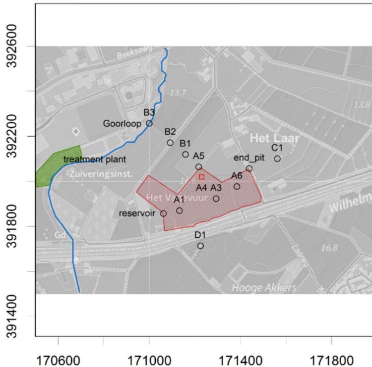
Figure 3.3: Monitoring network (points) for the Bavaria-case, where treated waste water from the Bavaria Brewery (green) is used for subirrigation of an and agricultural field (red).
