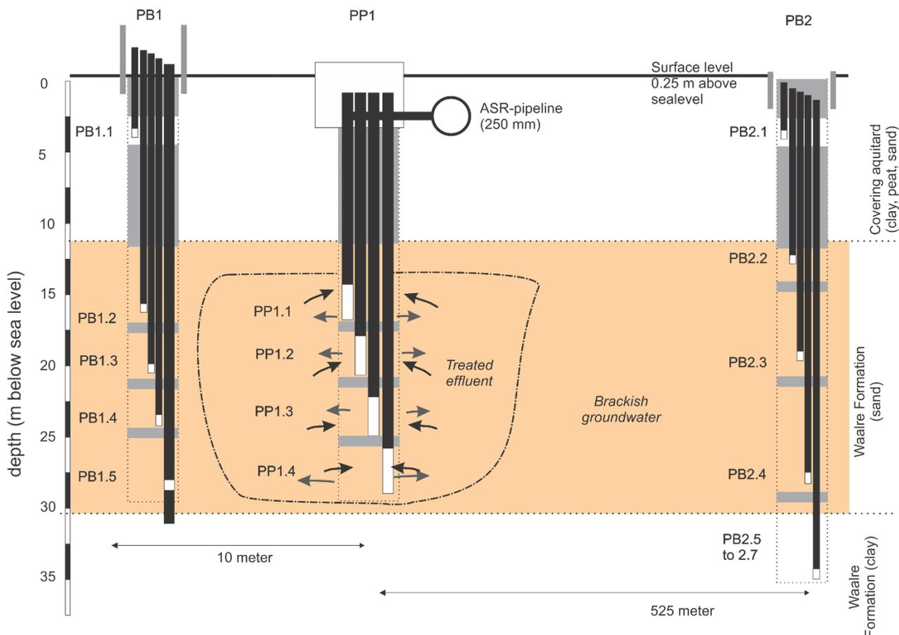
Figure 4-10: Cross-section of the ASR pilot at Dinteloord. PP1 is the ASR well.
