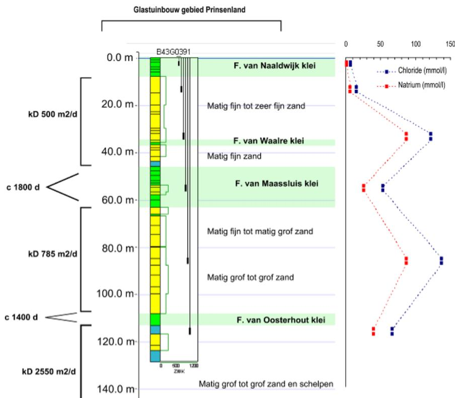
Figure 4-3: Hydrogeological schematization of the subsurface in the study area, including hydraulic parameters of discerned aquifers and aquitards and salinity distribution. Example of the content of the feasibility report (in Dutch).
