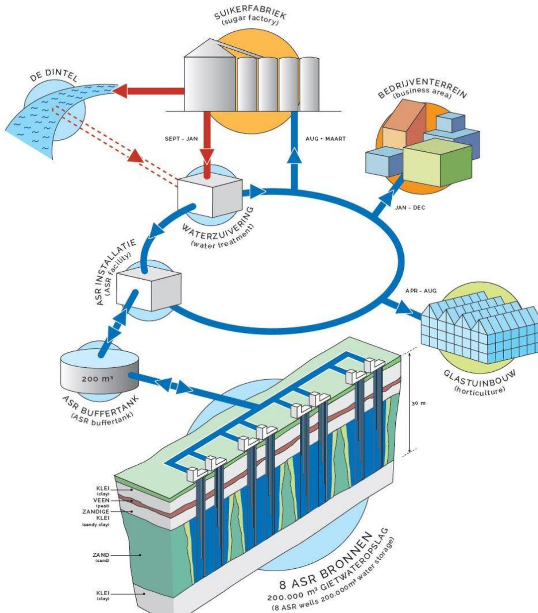
Figure 3-1: Set-up of the sustainable water supply system in Dinteloord
