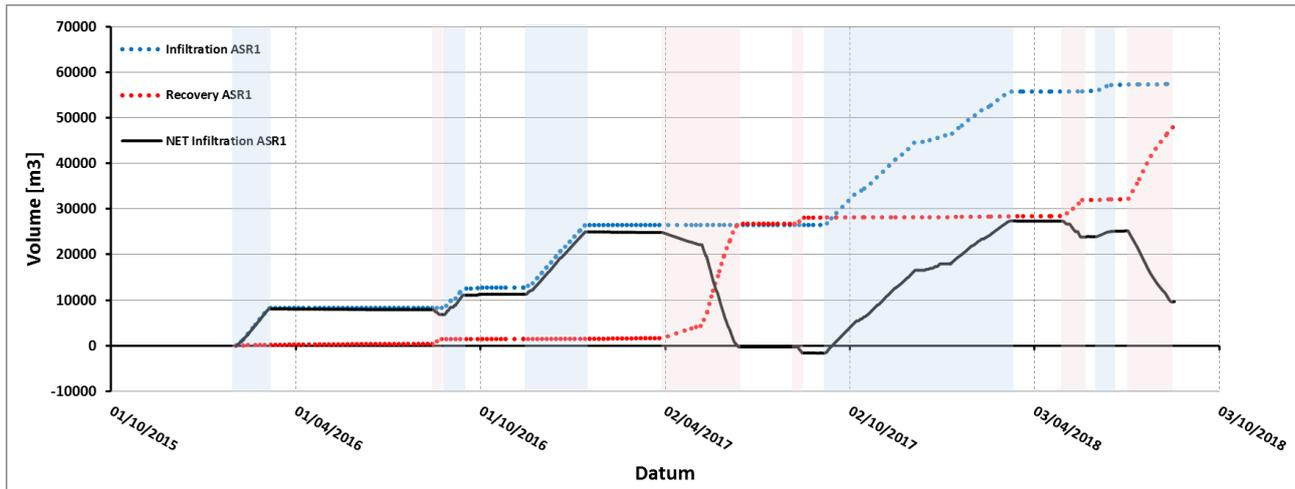
Figure A2-2: Infiltration (red dotted line and fields), recovery (blue dotted line and fields), and net infiltration (black solid line) of treated effluent through ASR1 from February 2016 till August 2018.
