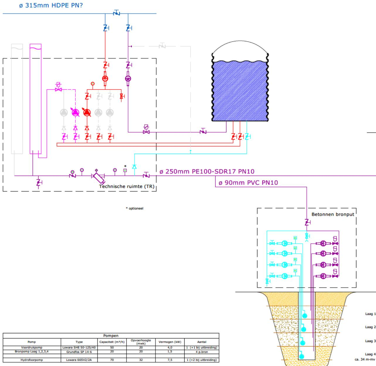
Figure 4-15: Brief technical overview of the water-system in Dinteloord, including the connection of the pilot ASR-well. A more detailed overview is given in Appendix 4. Example of drawings in the final design phase.
