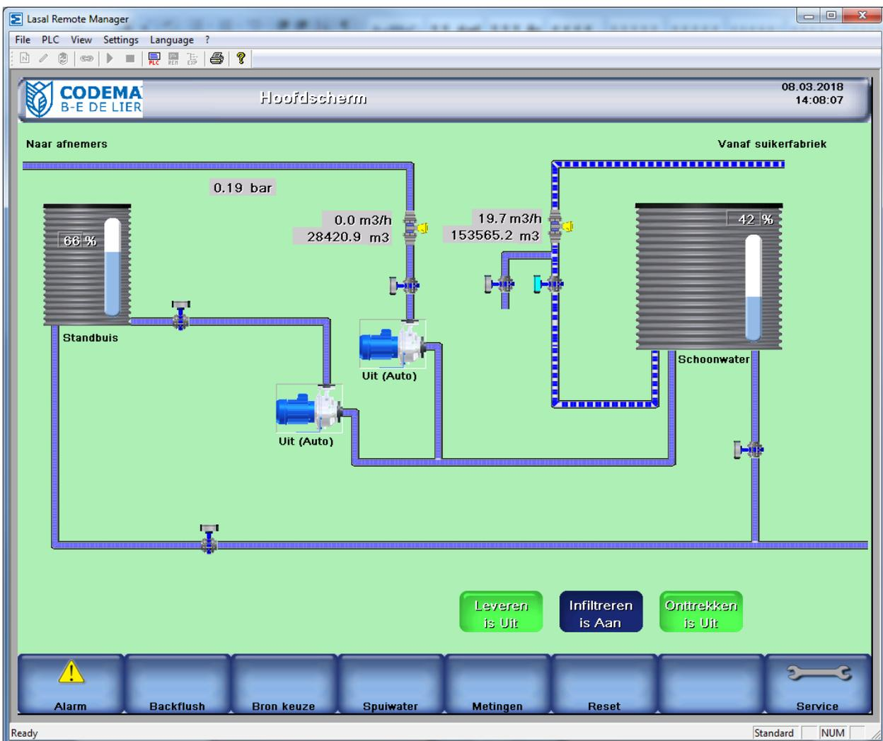
Figure 5-1: Main screen of the automated control unit of the watersystem in Dinteloord (in Dutch).
