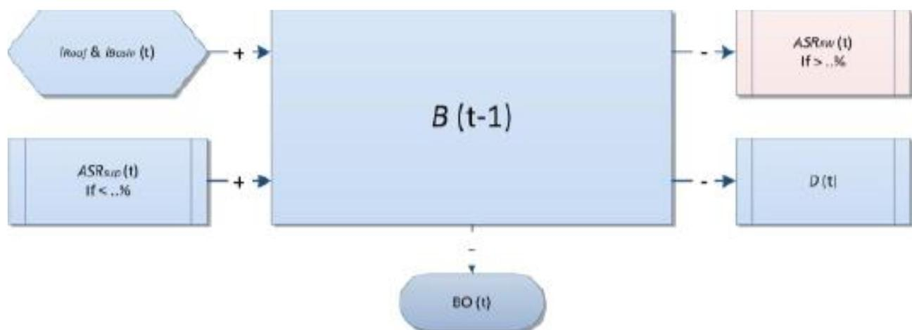
Figure A3-4: Simulation of the water volume in the surface storage basin.
