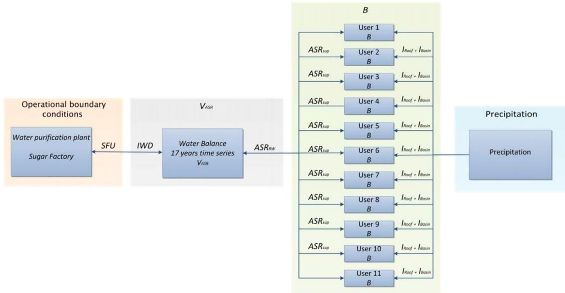
Figure A3-3: Lay-out of the water balance of Nieuw Prinsenland.
