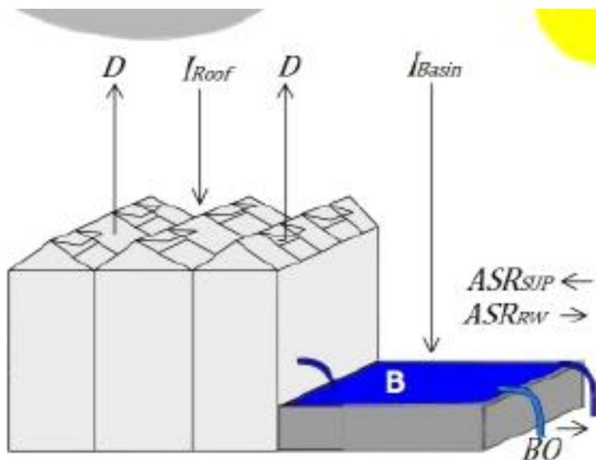
Figure A3-1: Schematic representation of the water balance of the greenhouse horticulturalists.
