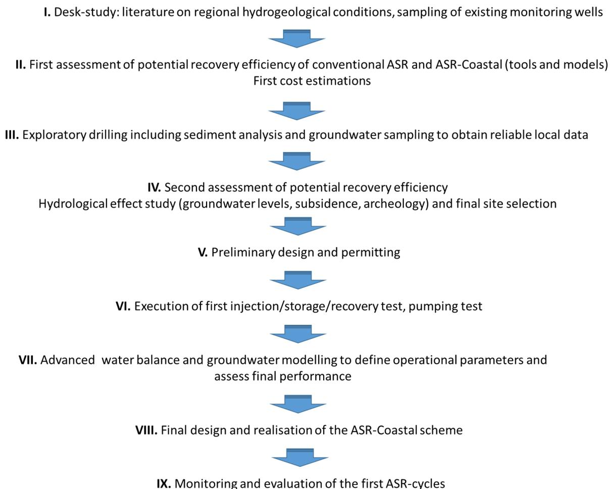
Figure 4-1: Stepwise approach to realize the ASR-Coastal scheme to enable water reuse in Dinteloord.
