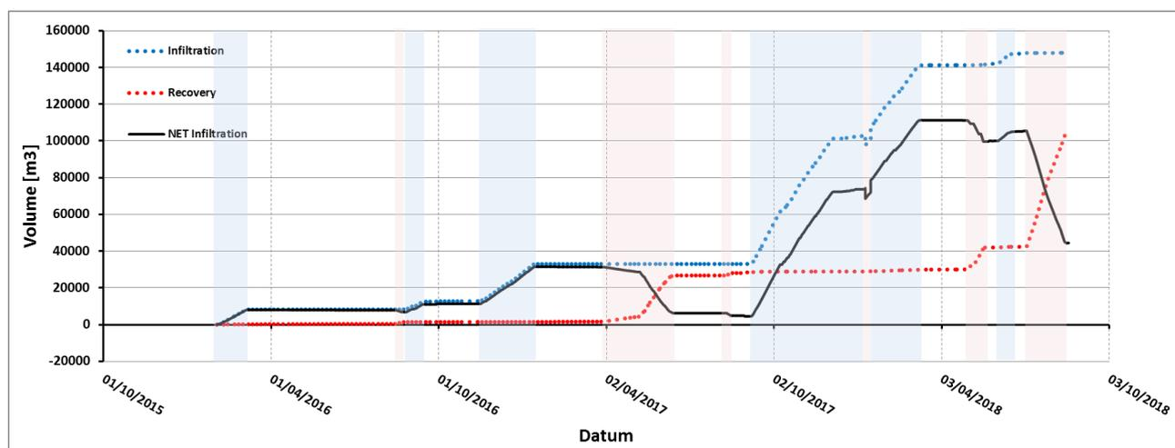
Figure A2-1: Infiltration (red dotted line and fields), recovery (blue dotted line and fields), and net infiltration (black solid line) of treated effluent through all ASR-wells from February 2016 till August 2018.
