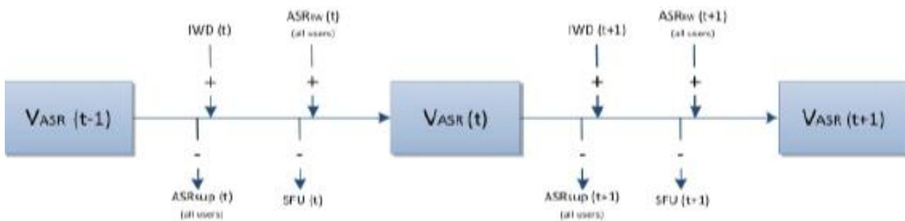
Figure A3-5: Simulation of the water volume stored in the subsurface.
