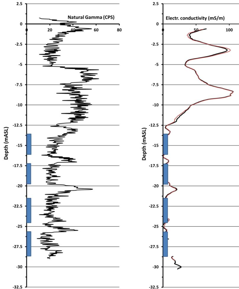
Figure A1-1: Natural gamma log and electrical conductivity at PB1 (Figure 4-13) on March 2016, after the first injection of freshwater. The blue rectangles represent the well screens of the first ASR well. The EC of the formation at the depth of these well screens is 0 mS/m, because treated effluent with a very low EC (<50  $\mu\text{S}/\text{cm}$ ) was already injected at the time of logging.
