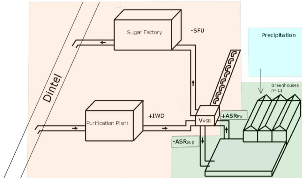
Figure A3-2: Schematic representation of the total water balance of Nieuw Prinsenland, with integration of the water balance of the greenhouse horticulturalists (green). For clarification: in this outline, waste water is first discharged to the river, after which intake of the same water occurs. This leads to a more constant water quality feeding the treatment.
