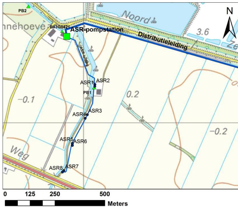
Figure 4-13: Overview of the final ASR facility in Dinteloord, including ASR-wells, monitoring wells, and infrastructure.
