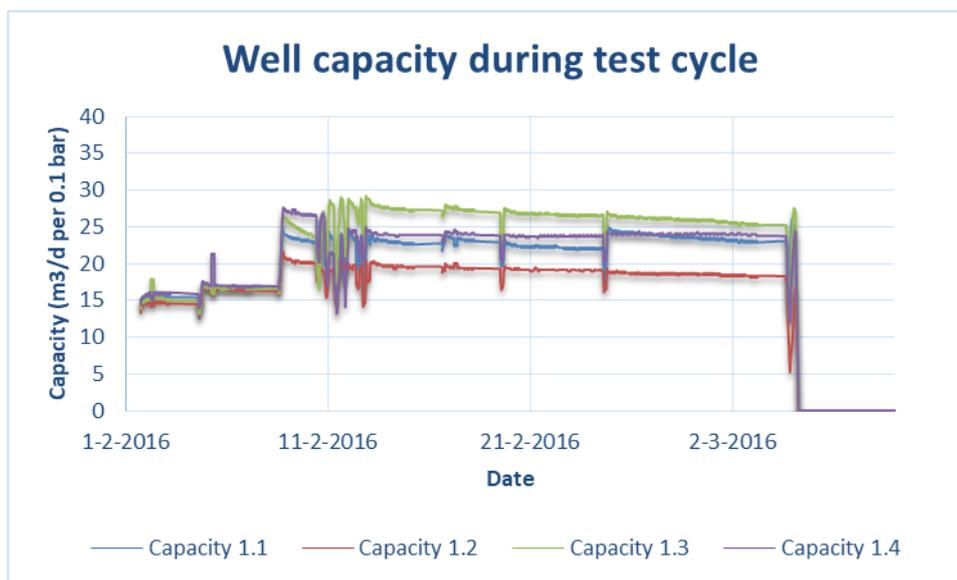
Figure 4-11: Example of the calculated well capacity (based on measurements) during the test cycle at the Dinteloord site.
