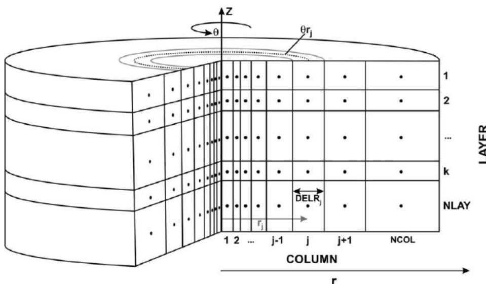
Figure 4-4: Set-up of an axi-symmetrical model based on Langevin (2008)
