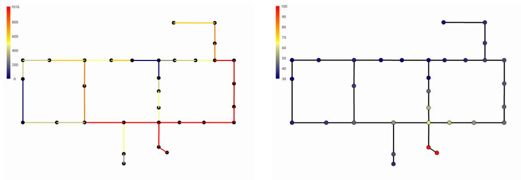
Fig. 10. a) Optimized diameters for the Hanoi benchmark. b) Corresponding nodal heads.
