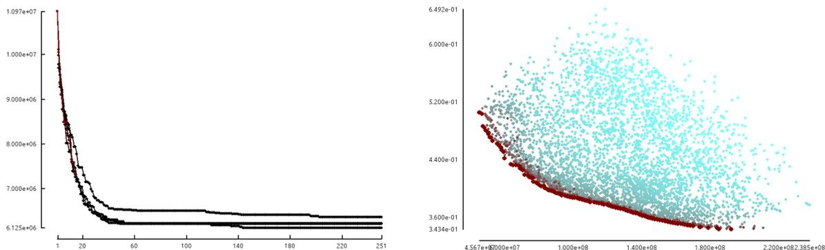
Fig. 7. Monitoring of progress during the optimization process: a) convergence curves for single or implicit multiobjective problems, b) Pareto front for explicit multiobjective problems.
