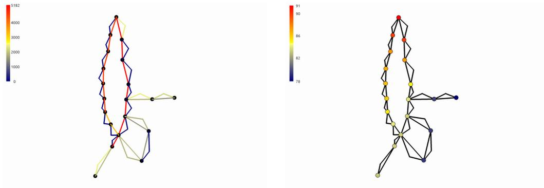
Fig. 9. a) Optimized diameters for the New York Tunnels benchmark. b) Corresponding nodal heads.
