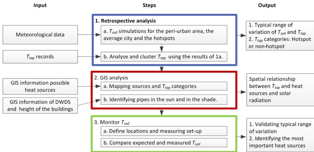
**Figure 1.** Proposed method to identify heat sources and urban characteristics that locally influence the soil temperature.
