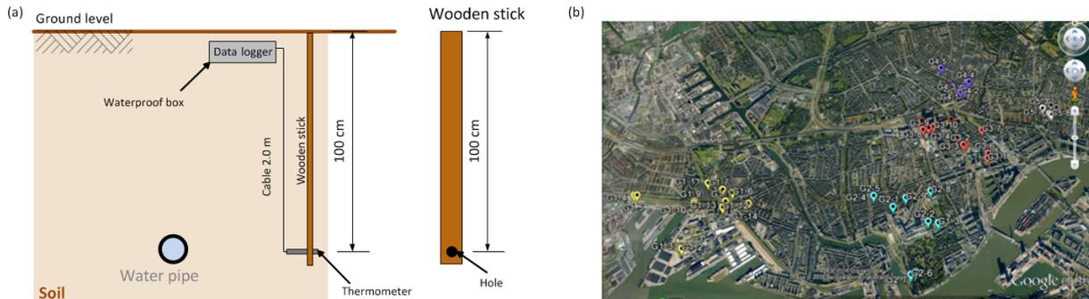
**Figure 4.** (a) Detail of the soil temperature measurement installation and (b) locations of the measurements (source: Google Earth).
