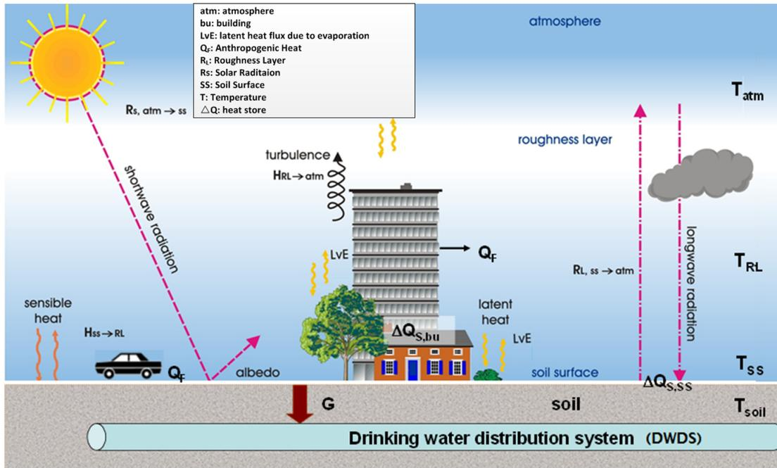
Figure 2. Schematic heat transfer in an urban setting (following Blokker and Pieterse-Quirijns, 2013).
