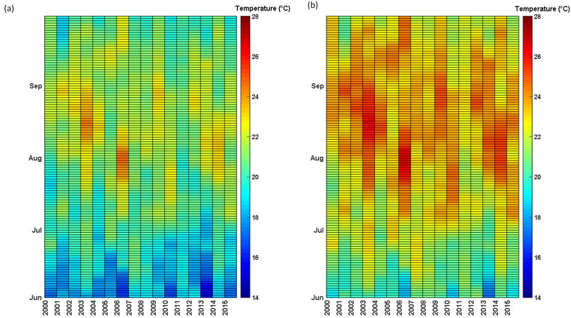
**Figure 5.** Simulations of  $T_{\text{soil}}$  at  $-1.0$  m in the average city (a) and in the hotspots (b) from 2000 until 2015 during the months June, July, August and September.
