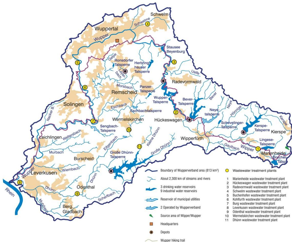
**Figure 7. Main hydraulic structures and water bodies in the Wupper River Basin**
