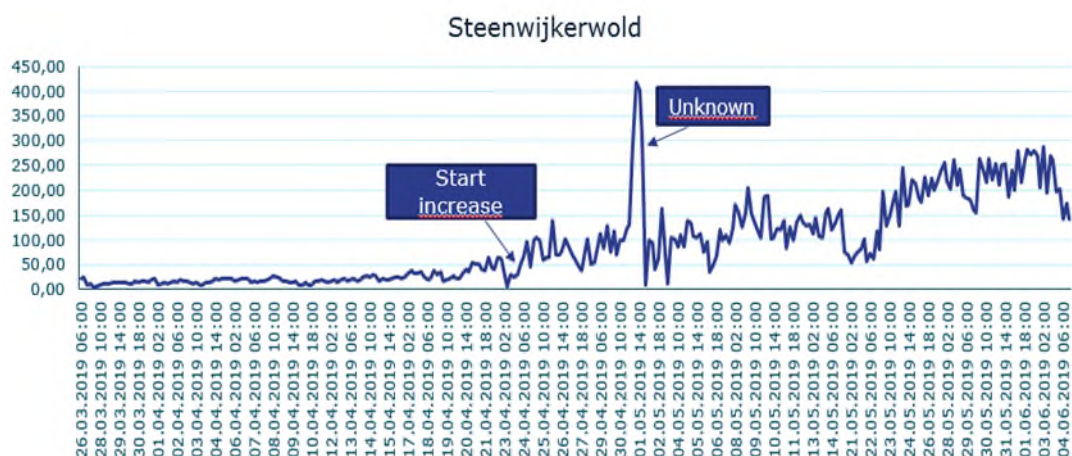
Figure 58. Enzymatic activities (measured with the BACTcontrol) in the outgoing water to Steenwijkerwold
