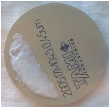
Figure 7. Filter of the BACTcontrol after measuring cooling tower water. A white, slimy layer is present on the lower side of the filter.
