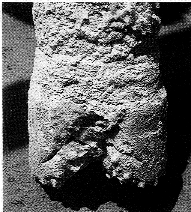
Figure 6. Drill bit covered with frozen mud after water invaded the borehole.
