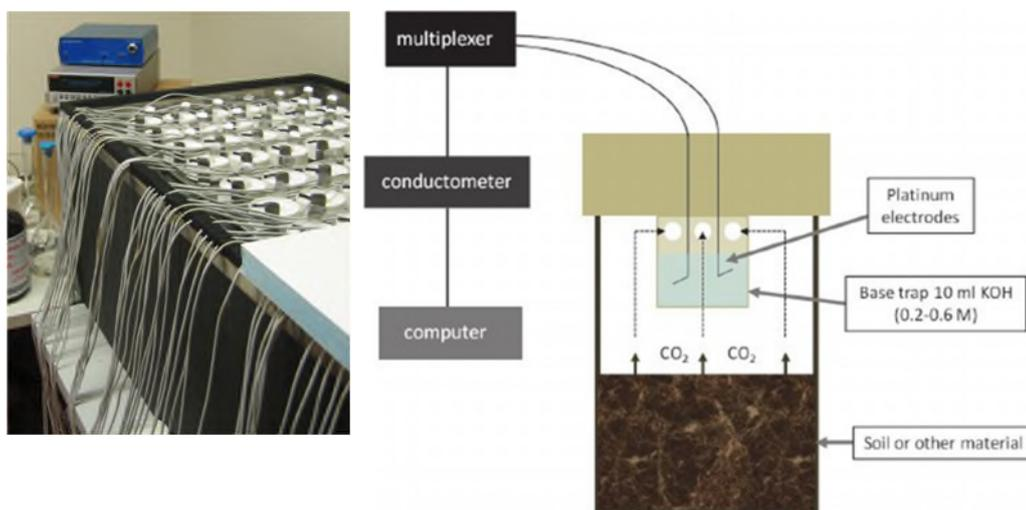
Figure 12. Left. Example of Respicond V installation (<http://www.respicond.com>). Right: Individual Respicond measurement cell (Kainiemi, V., 2014)
