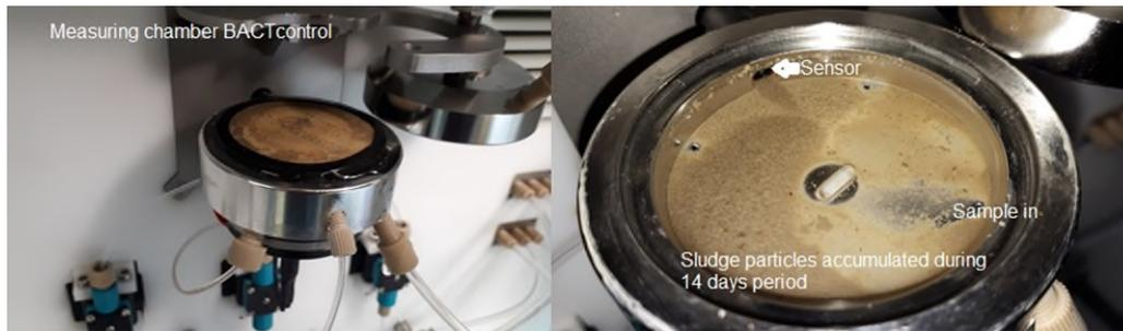
FIGURE 31. STATUS OF MEASURING CHAMBER BACTCONTROL DURING MAINTENANCE AFTER A RUN PERIOD OF 14 DAYS.
