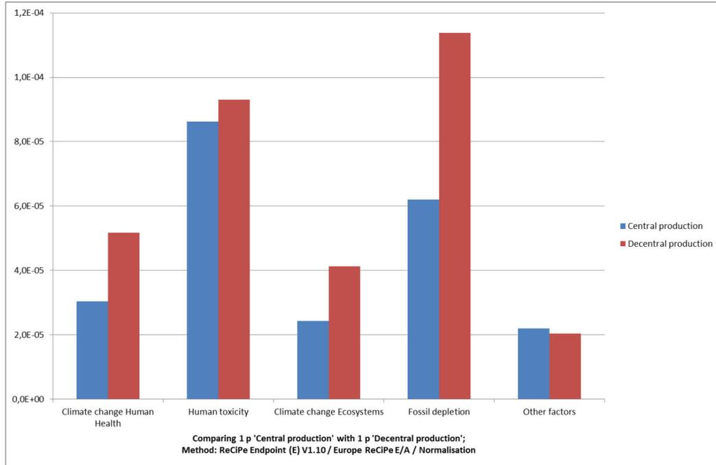
FIGURE 11 THE COMPARISON OF ENVIRONMENTAL IMPACT OF CENTRALISED AND DECENTRALISED DRINKING WATER PRODUCTION
