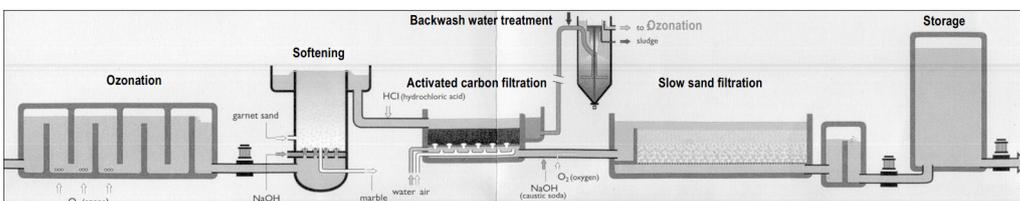
FIGURE 7 SCHEMATIC OVERVIEW OF DRINKING WATER PRODUCTION AT WEESPERKARSPEL
