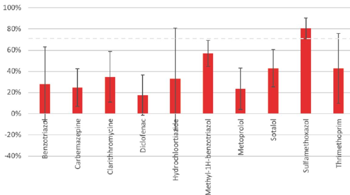
Figure 2- Removal rate of OMPs at the WWTP of Aarle- Rixtel, in a total of 10 composite samples, collected during a 24h period. The monitoring period was from 10 May to 27 June, 2019. Propranolol was monitored, but the concentrations were below detection level (Source: Nieuwenhuis et al. (2021)). The added dotted line indicates the target of 70% OMP removal, proposed by the *Ministerie I&W*.
